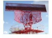
**RL 2000** – Latest generation of ELDIS primary surveillance radars for Terminal Approach Control Application. The RL-2000 design is benefiting from the long time experience on several civilian and military radar types. The radar meets or exceeds ICAO and EUROCONTROL recommendations and standards. The RL-2000 features fully solid-
