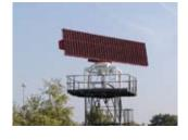
MSSR Radar – Monopulse Secondary Surveillance Radar developed by company ELDIS is fully modular, meets ICAO standard and is delivered in basic configuration, extendable for S-mode function. Basic configuration of the autonomous secondary radar fully comply with standard MARK X and allows extension according to increasing needs
